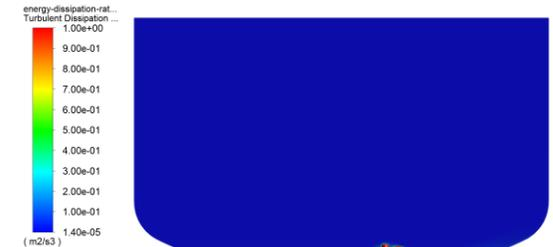
Energy dissipation rate per mass unit for the new 500 liters tank at 225 rpm
