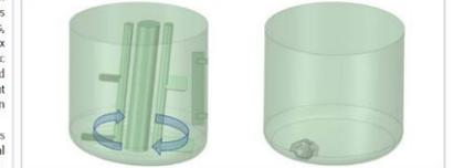
Fig. 12.a: Existing 100 liters tank with paddle mixer. Fig. 12.b: New 100 liters tank with GM1 NovAseptic<sup>®</sup> mixer.
